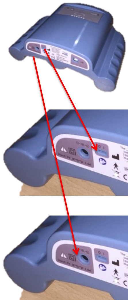
Location of power socket
