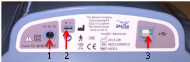
Figure 5: Connections on the lower side
