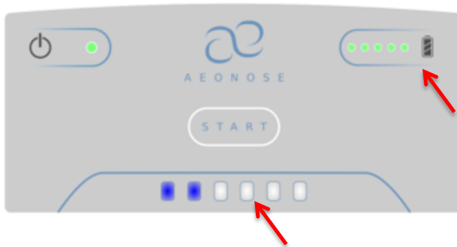
Figure 4: process indicator LED's and battery indicator
